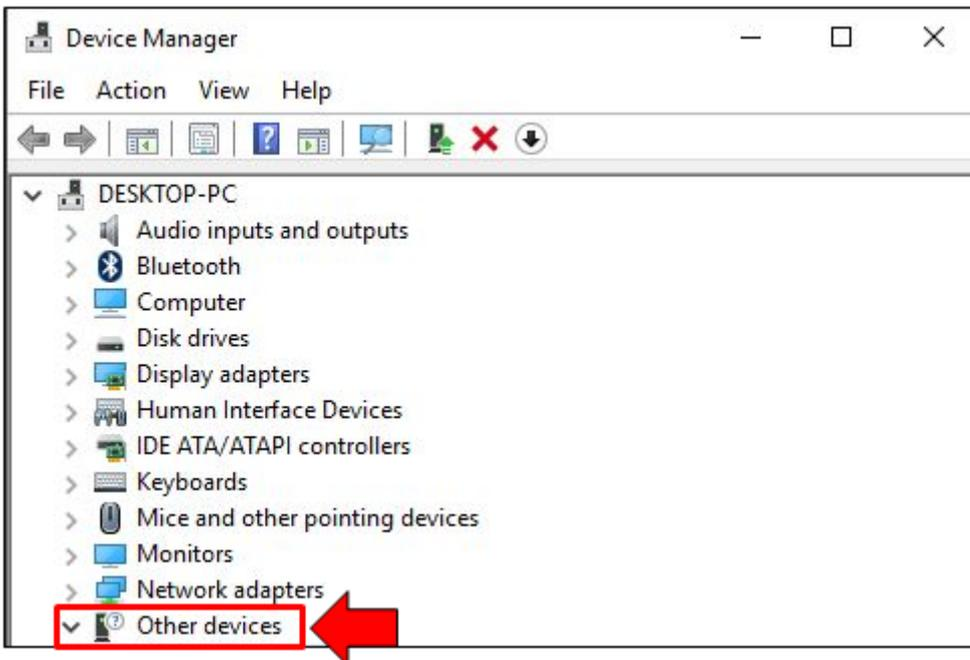
Clicking on this ***“Other devices”*** item from the list will cause it to expand and show all the hardware that currently don’t have the proper driver for them to work. These devices should be labelled as ***“Unknown device”*** as shown below and its icon should have a yellow triangular overlay on it that contains an exclamation mark in it.
